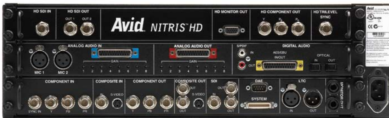
Avid DS Nitris system features a broad range of professional input/output connections, including analog video and audio.
